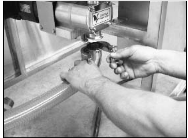
30. Remove the lower glaze hose clamp and gasket.
